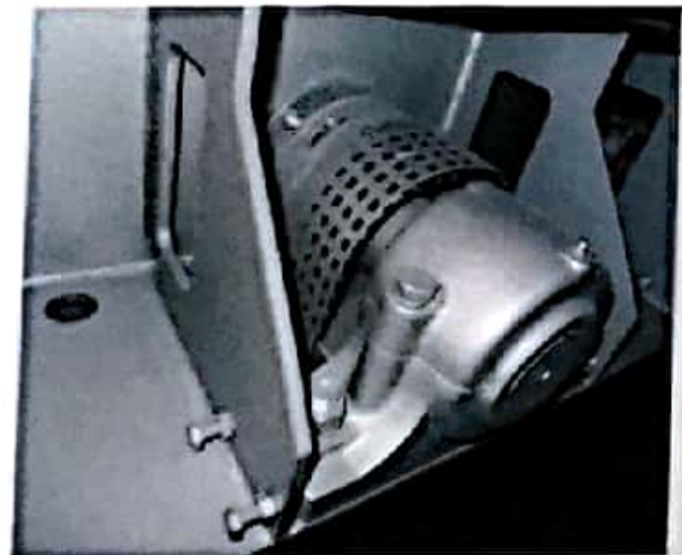
平衡组合密封 Counter Balance Seal Assembly For Main Shaft (with Patent Certificate)
