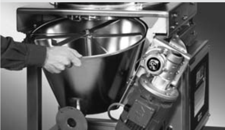
Removing feed hopper
