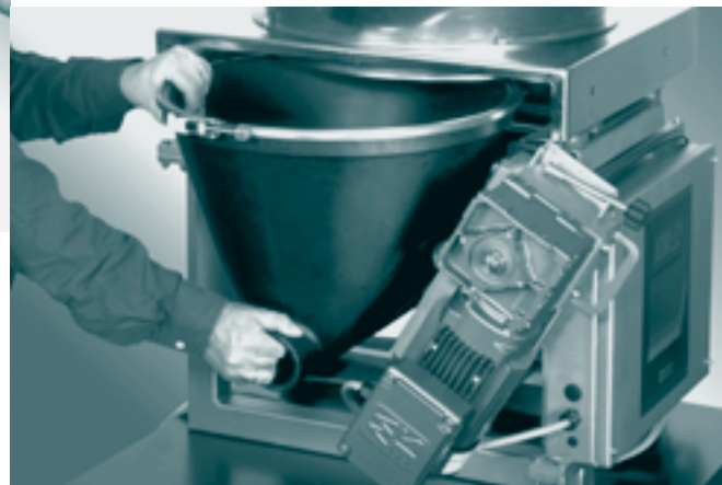
Removing feed hopper
