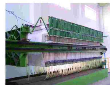
滤布曲张机构 Vibrate cloth device
