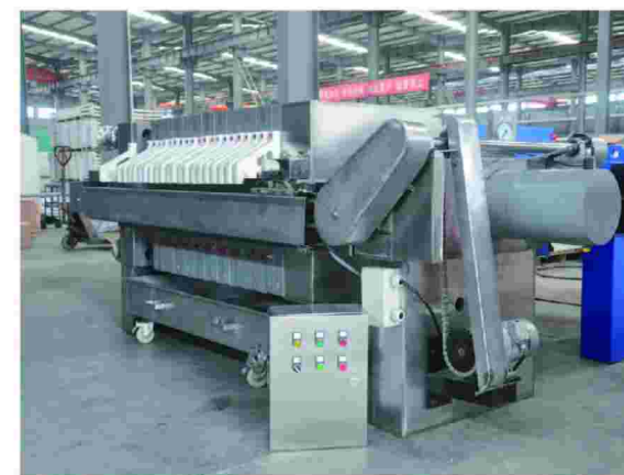
带移动料斗压滤机 Filter press with moveable cake trolley
