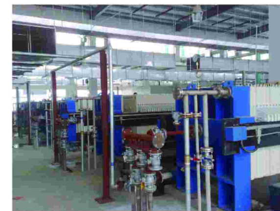
化工行业压滤机 Filter press applied in chemical industries
