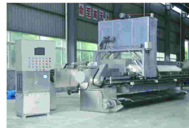
▲ 双杆水洗 double pole wash cloth
