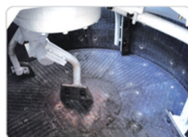
堆焊衬板 / Hard surfacing material liner
